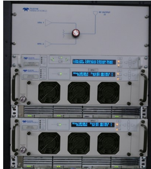
125W Ku-Band 1:1 Redundant System in the 3RU Chassis, with N+1 redundant power supplies
