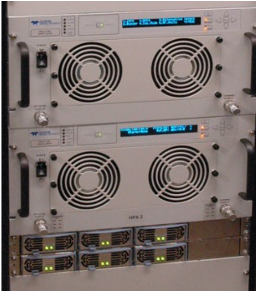
600W C-Band, 1:1 Redundant System in the 5RU chassis, with N+1 redundant power supplies
